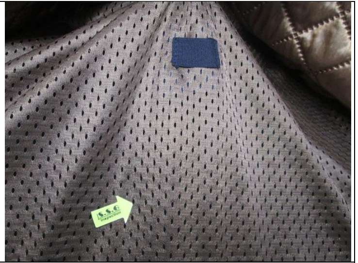
Like this one. Style / STROKER You can see missed joint stitch.
