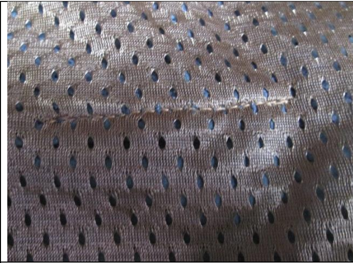
Like this one. Style / STROKER You can see missed joint stitch.
